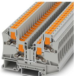
Feed-through terminal block, nom. voltage: 1000 V, nominal current: 41 A, connection method: Push-in connection, Rated cross section: 6 mm<sup>2</sup>, cross section: 0.5 mm<sup>2</sup> - 10 mm<sup>2</sup>, mounting type: NS 35/7,5, NS 35/15, color: gray
