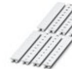
Zack marker strip, Strip, white, labeled, can be labeled with: CMS-P1-PLOTTER, printed horizontally: consecutive numbers 1 ... 10, 11 ... 20, etc. up to 91 ... 100, mounting type: snap into tall marker groove, for terminal block width: 8.2 mm, lettering field size: 10.5 x 8.15 mm, Number of individual labels: 10
