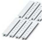
Marker for terminal blocks, Strip, white, labeled, can be labeled with: CMS-P1-PLOTTER, horizontal: L1, L2, L3, N, PE, L1, L2, L3, N, PE, mounting type: snap into tall marker groove, for terminal block width: 8.2 mm, lettering field size: 10.5 x 8.15 mm, Number of individual labels: 10
