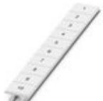
Zack marker strip, Strip, white, labeled, can be labeled with: CMS-P1-PLOTTER, Printed vertically: consecutive numbers 1 ... 10, 11 ... 20, etc. up to 91 ... 100, mounting type: snap into tall marker groove, for terminal block width: 8.2 mm, lettering field size: 10.5 x 8.15 mm, Number of individual labels: 10
